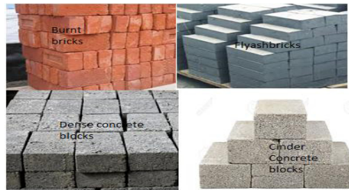
Fig. 2. Images of different building wall materials
