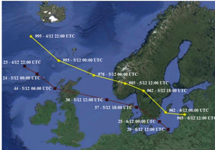
Fig. 4. Mean sea level pressure in hPa (yellow) and maximum WPD in \text{kW/m}^2 at 100 m (red) tracks for cyclone Xaver as simulated by WRF model.
