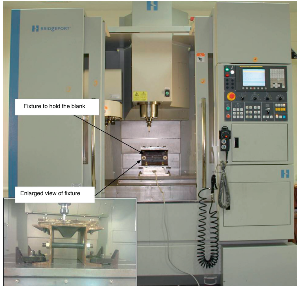
Fig. 5 – Experimental setup for incremental forming on CNC milling machine.
