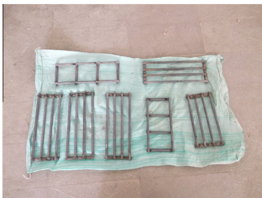
Figure 2 Shape of swimmer bar planes.
