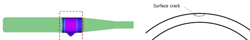
Fig. 7. Mooring anchor pile and surface crack.
