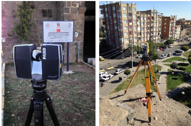
Figure 3. FARO Laser Scanner and TotalStation.
