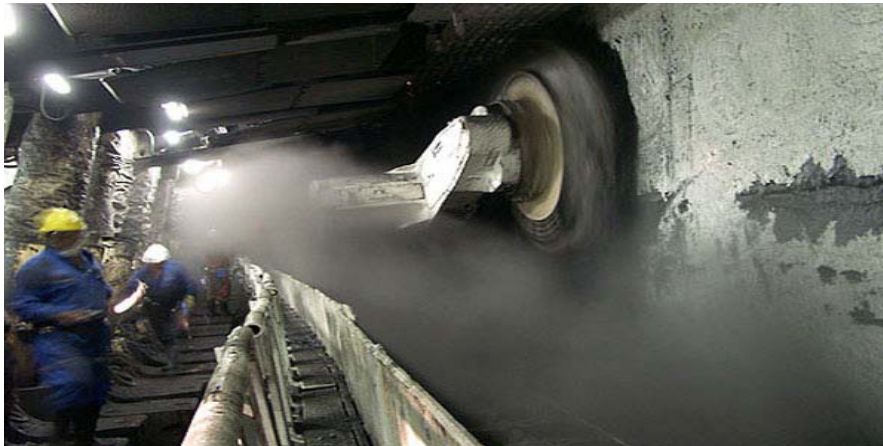
Fig. 2. Dust generation with shearer
