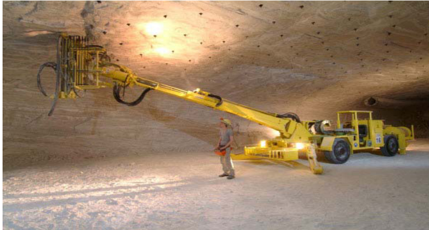
Fig. 4. Automated temporary roof supporter
