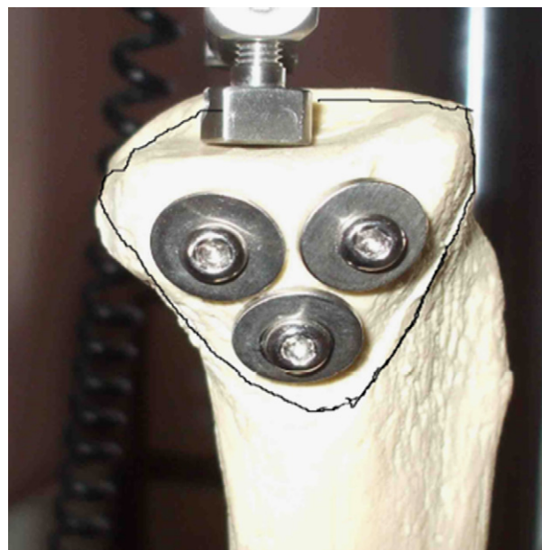
Figure 2 Fixation with three 6.5 mm cancellous screws.
