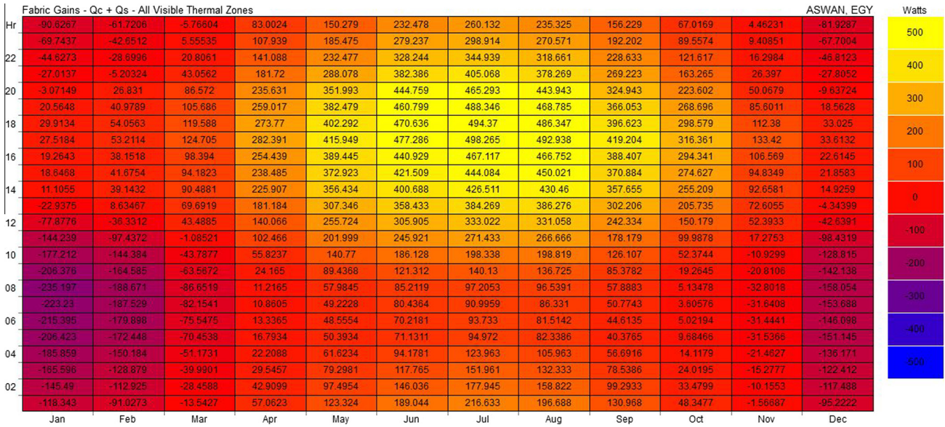
Figure 8. Rates of fabric heat transfer through the envelope of the baseline model B – Paints and coatings.
