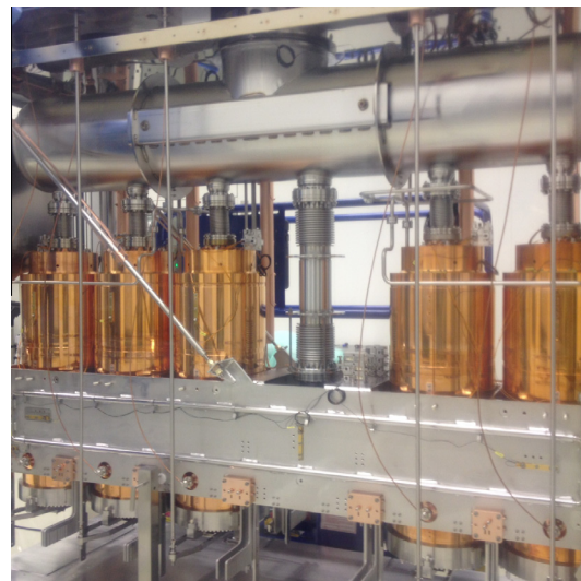
Fig. 5. Photo of the elements inside the cryo-module vessel and thermal shield, the five cavities clearly visible.
