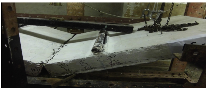
Figure 4 Brittle failure of slab AS-3.
