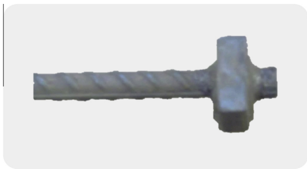
Figure 1 Shape of the prepared headed bar after welding.
