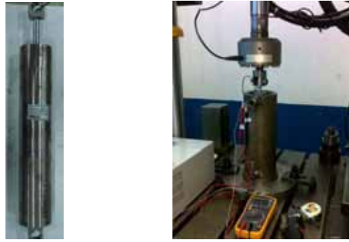
Fig.5. (a) MR damper Sample Piece (b) Experiment Frock
