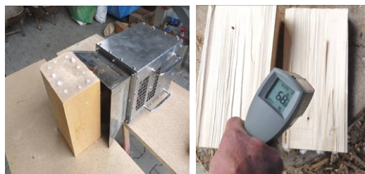
Fig. 6. Presentation of experimental sterilization of wood-destroying insects (author)
