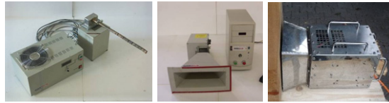
Fig. 4. Photos of drying microwave device (author)
