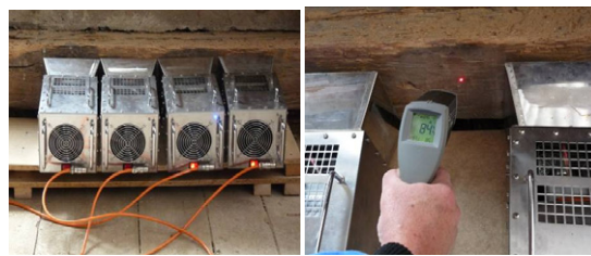
Fig. 7. Presentation of experimental sterilization of wood-destroying insects “in situ” (author)
