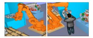
Fig. 2: Illustration of a conceptual model of a collaborative assembly cell. The operator is responsible for guiding the robot to the correct location. The robot is used as a flexible lifting device [4].
