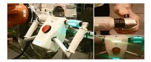
Fig. 3: A concept for a hand-guiding device that can used to move the flywheel housing cover (left) into position. A switch that increases the accuracy of robot motion to enable precise assembly (Right Top). The yellow indicator light conveys to the operator that the guiding pins are engaged and that the cover can be released. (Right Bottom).
