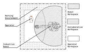
Fig. 1: Illustration of the interaction between the three participants of a collaborative assembly cell within their corresponding workspaces.
