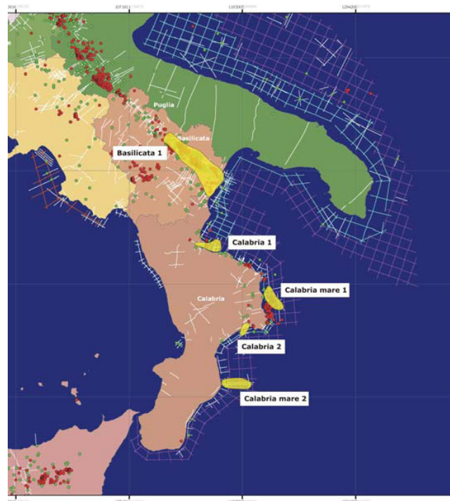
Figure 3 Map of most promising areas for geological storage in Italy (Donda et al, 2008)
