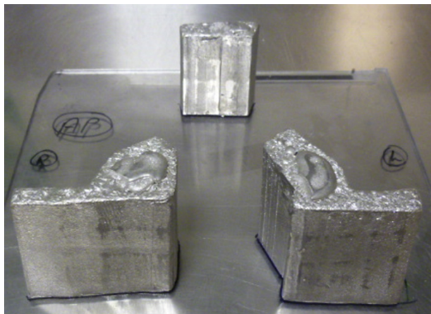
Figure 2. Blocks used for beam shaping. These hand-poured metal blocks are placed into the treatment machine to attenuate the beam in selected areas.
