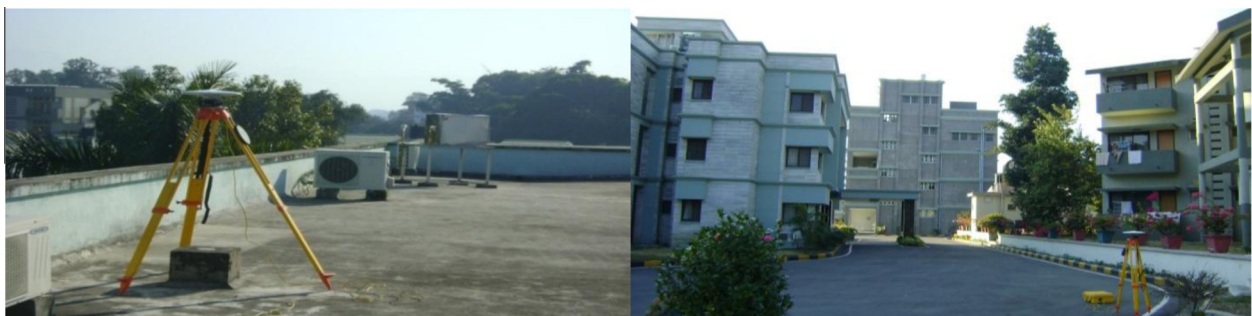
Figure 1 GPS antennas (a) Base receiver on top of building (b) Rover at test site (Trimble R7 GNSS Base & Rover).
