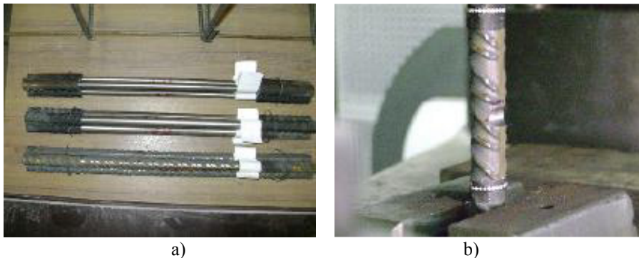
Fig. 3. a) Rebars abraded concentrically. b) Damaged rebar locally abraded.
