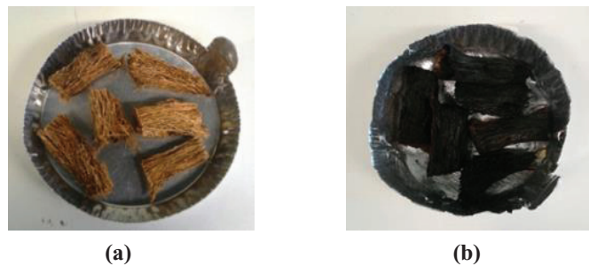
Fig. 3. Appearance of EFB (a) before and (b) after torrefaction in combustion gas.
