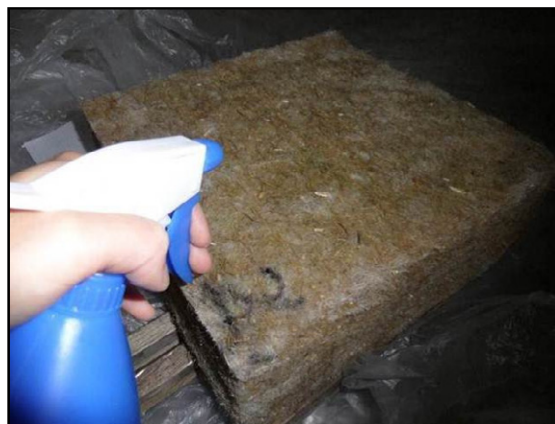
Fig. 3. Application of hydrophobic substance – spray
