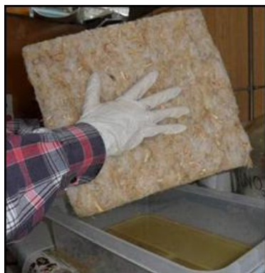
Fig. 2. Application of hydrophobic substance – soaking
