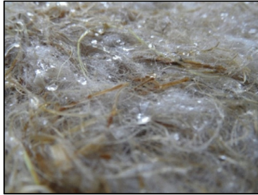
Fig. 7. Test sample TG after short-term absorbability test
