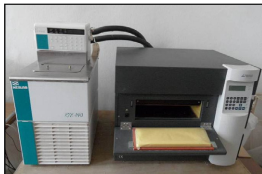
Fig. 5. Testing apparatus for determination of thermal conductivity
