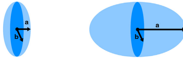
Fig. 3. Oblate (left) and prolate (right) ellipsoid and the corresponding radii. The movement of ellipsoids in the fluid is from left to right.
