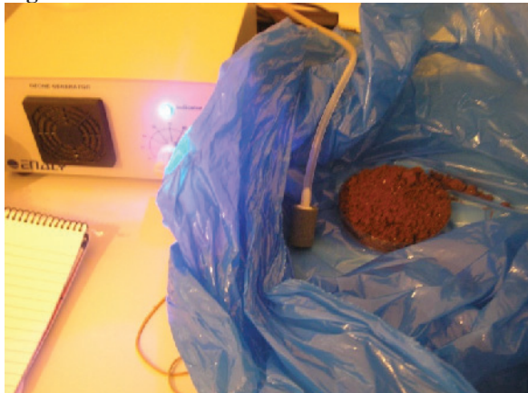
Figure 3: Soil fumigation with O_3 gas
