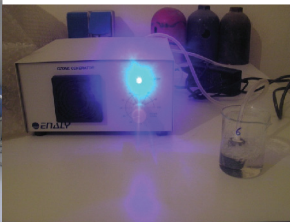
Figure. 2: Ozone generator & direct ozonation
