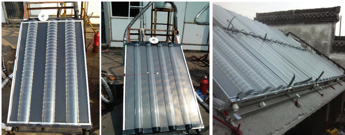
Fig.3. collectors with 2 types of PMMA covers and tile-shaped collectors mounted on the pitched roof
