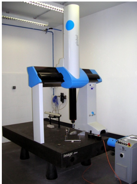
Fig. 1. Moving bridge coordinate measuring machine used in the present study.
