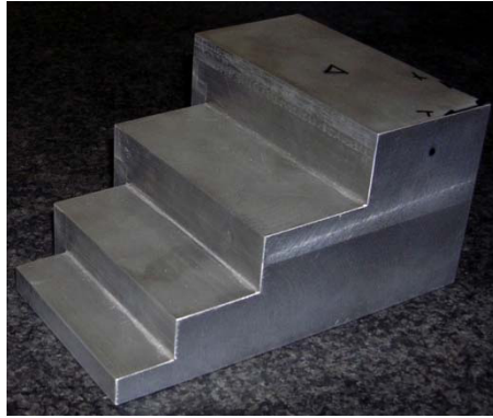
Fig. 3. Machined part to be measured with both contact probes: TP-200 and SP-25.
