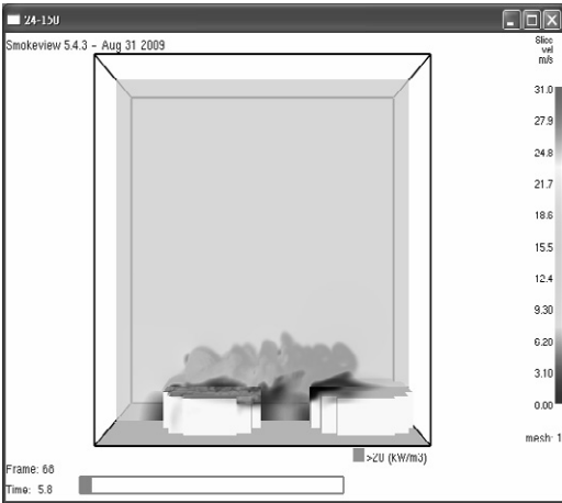
Figure 6. About 6 seconds after the fire effects of wind speed on fire
