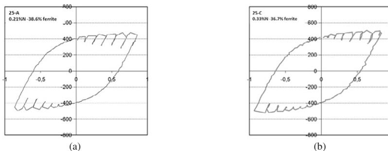
Fig. 2. Response jagged curves from the 2<sup>nd</sup> cycles for Alloy 25-A and Alloy 25-C during cyclic loading at 350°C.
