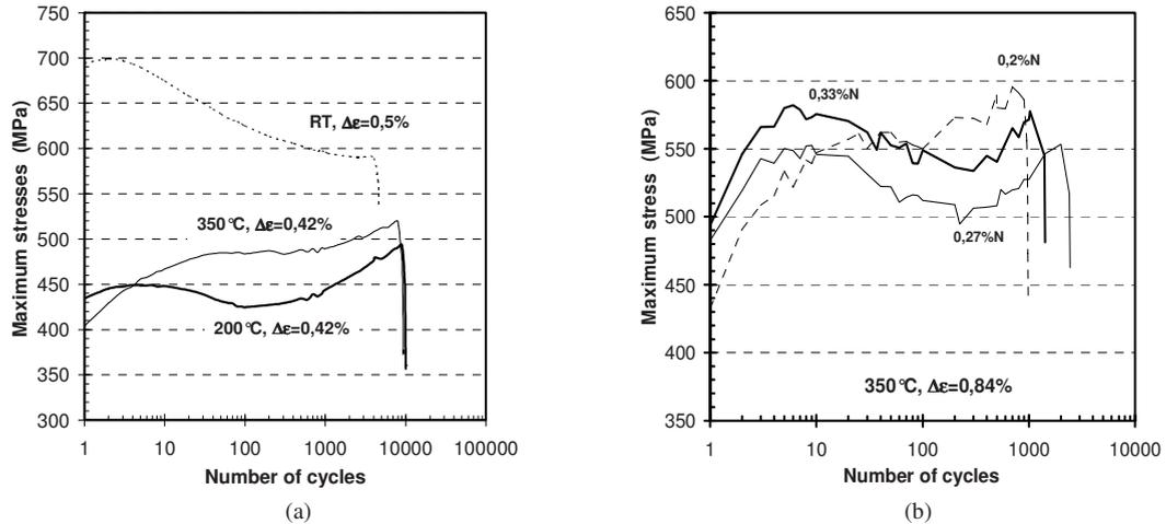
Fig. 1. Stress response curves in modified super duplex stainless steel S32705 grades, (a). Influence of temperature; (b). Influence of nitrogen contents.
