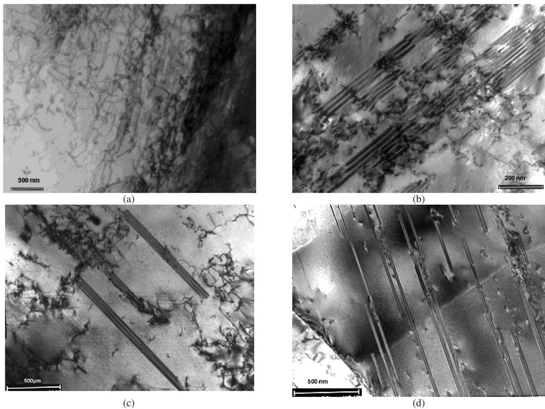
Fig. 3. Dislocation structures, (a). Planar dislocation in the austenitic phase,  $\Delta\epsilon/2=0,6\%$ , 4608 cycles, at RT; (b). Interaction between dislocations and stacking faults in the austenitic phase,  $\Delta\epsilon/2=0,84\%$ , 2456 cycles, at 350°C; (c). 0,21%N, austenite,  $\Delta\epsilon/2=0,84\%$ , 1486 cycles, 350°C; (d). 0,33%N, austenite,  $\Delta\epsilon/2=0,84\%$ , 1417 cycles, 350°C..
