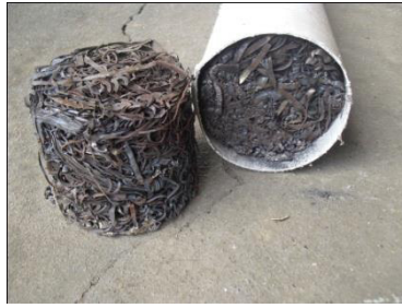
Fig. 2. Annealed and compacted billet of steel waste chips as desulfurizer.
