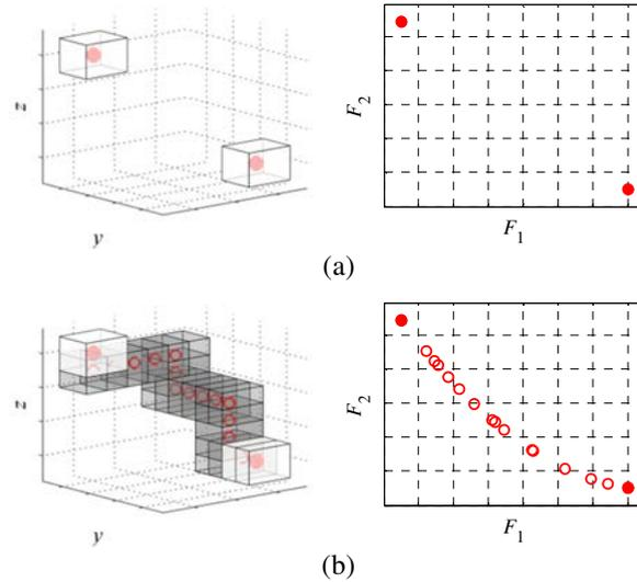
Fig. 1. A conceptual illustration of SDP algorithm ( $n = 3$ ): (a) “extreme” Pareto designs obtained from (1) ( $\bullet$ ); (b) SDP-based Pareto-optimal solutions ( $\circ$ ). Left- and right-hand side figures represent path in the design space and the feature space, respectively.
