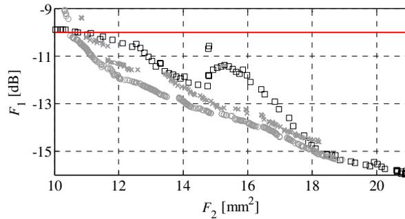
Fig. 5. Comparison of initial Pareto fronts obtained using SDP (○), as well as first (□) and second (×) benchmark method.
