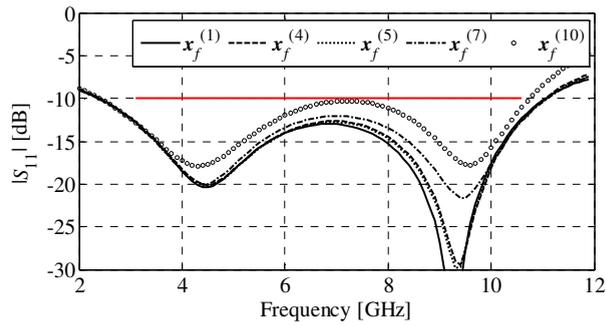
Fig. 4. Frequency characteristics of the transformer designs of Table 1.
