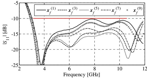
Fig. 8. Frequency characteristics of transformer designs of Table 2.
