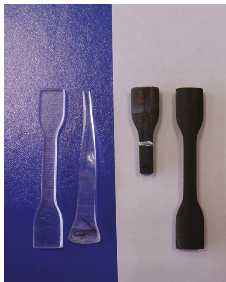
Fig. 3. Necking behaviour observed in neat polymer aged to low dose (white samples). The total recovery in industrial EPDM (black samples).
