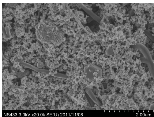
Fig. 2. A SEM photograph of the surface of a virgin \text{LiMn}_2\text{O}_4 cathode
