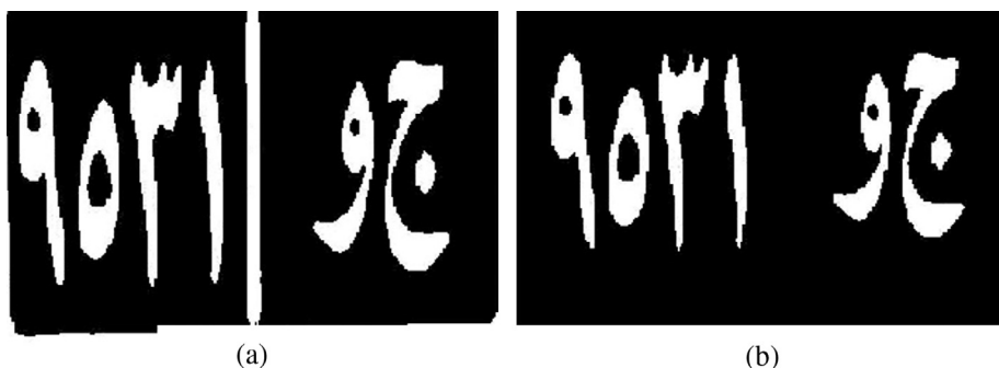
Figure 8 (a) Image with outer border. (b) Image without border.
