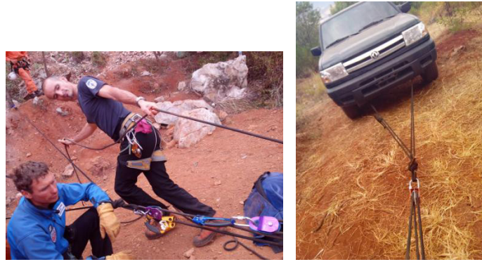
Fig. 6. The “rope pulley traction technology”
