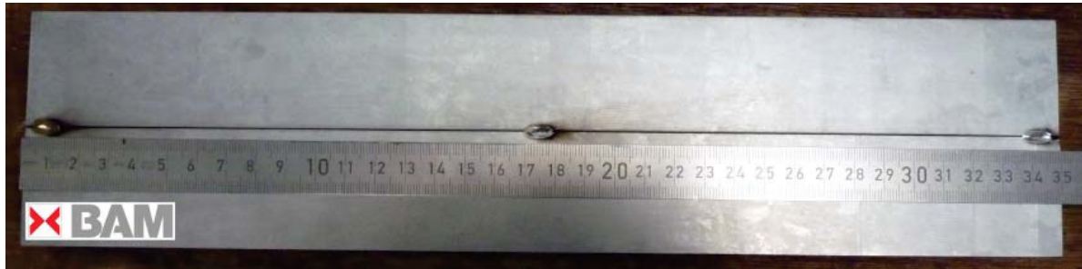
Fig. 1. Dimensions of the Ti3Al2.5V workpiece with a thickness of 16 mm.
