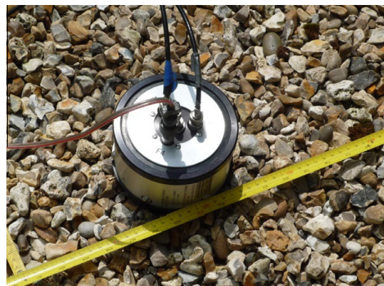
Fig. 5. Electrodynamic shaker (here on a gravel surface).
