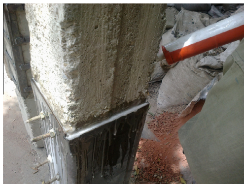
Fig. 4 Injection of tested specimens.
