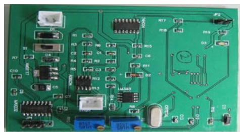
Fig. 7. circuit board of amplifier unit, comparison unit, plus detection unit and power unit.
