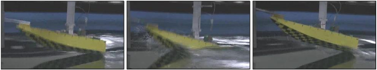
Fig. 14 Snapshot of VPS model at F_n = 1.44 (wave length : 6.0 L ).
