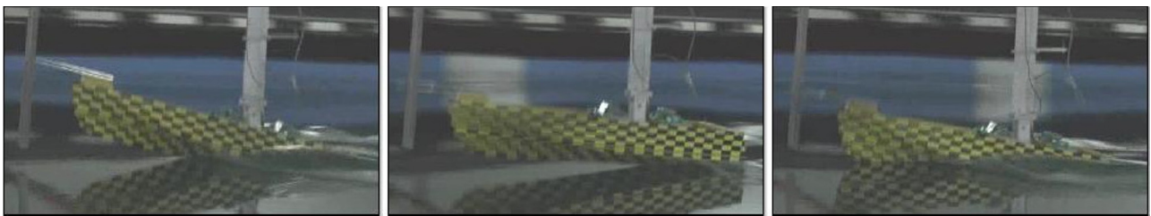
Fig. 16 Snapshot of VWS model at F_n = 1.44 (wave length : 4.5 L ).
