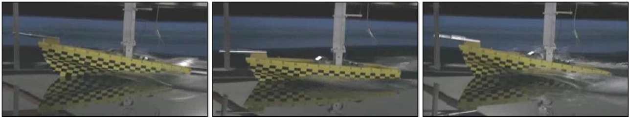
Fig. 15 Snapshot of VWC model at F_n = 1.44 (wave length : 5.0 L ).
