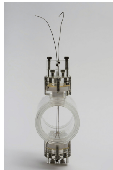
Fig. 2. Photograph of the 2-mm double-wire, conductance probe.
