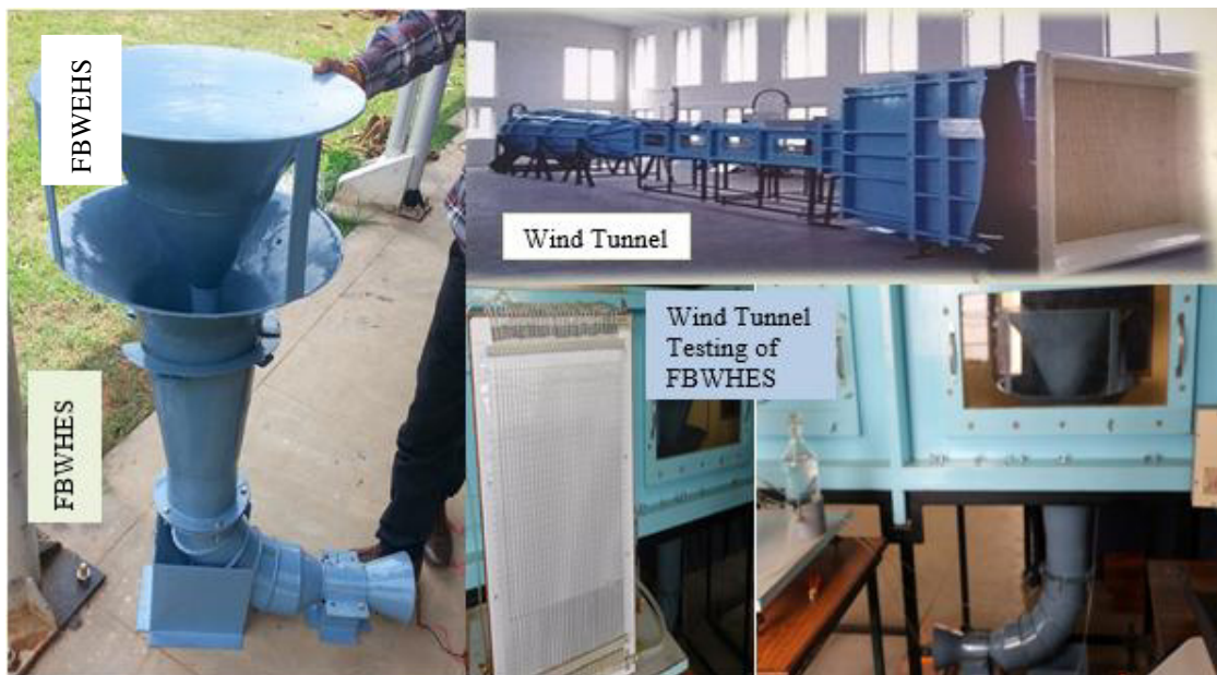
Fig. 4. Experimental setup of FBWEHS and wind tunnel testing
