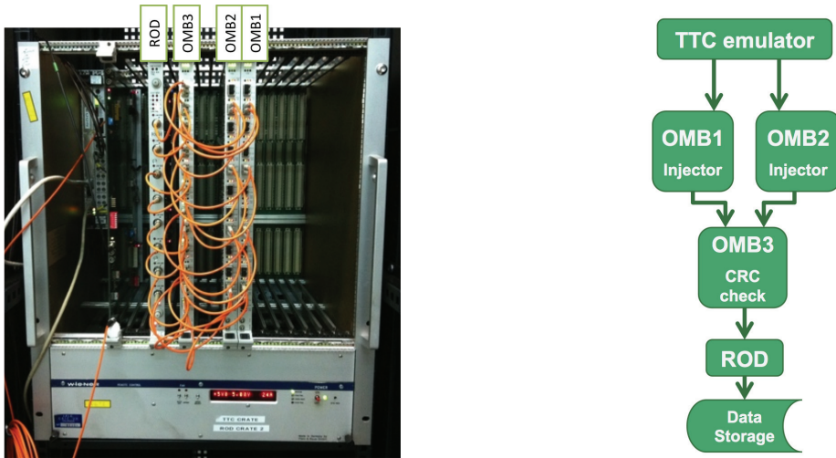
Fig. 4. (a) Picture of the OMB production crate with three OMBs and a ROD module; (b) Sketch of the qualification test-bench.
