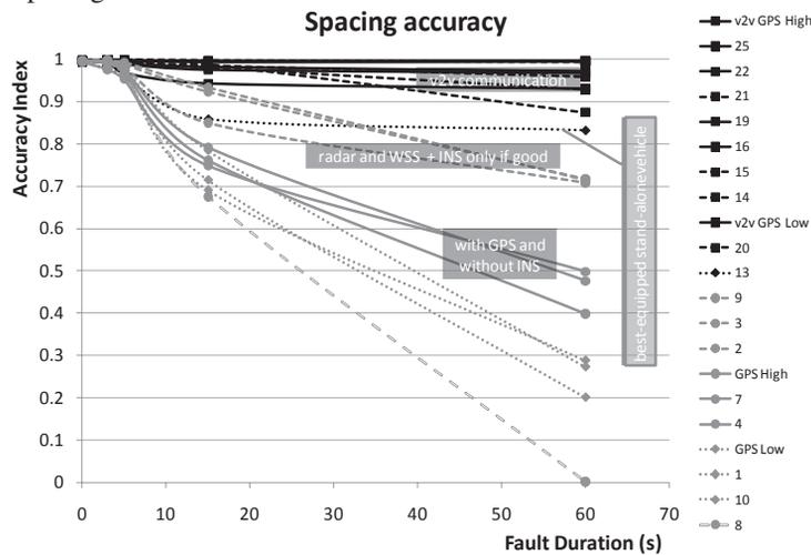
Figure 4 – Accuracy in reproducing spacing in case of radar fault
