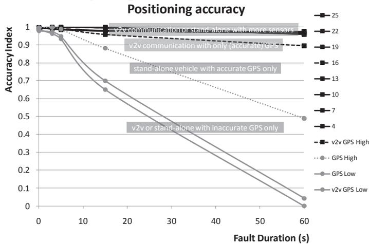
Figure 5 – Accuracy in reproducing positioning in case of both radar and GPS fault
