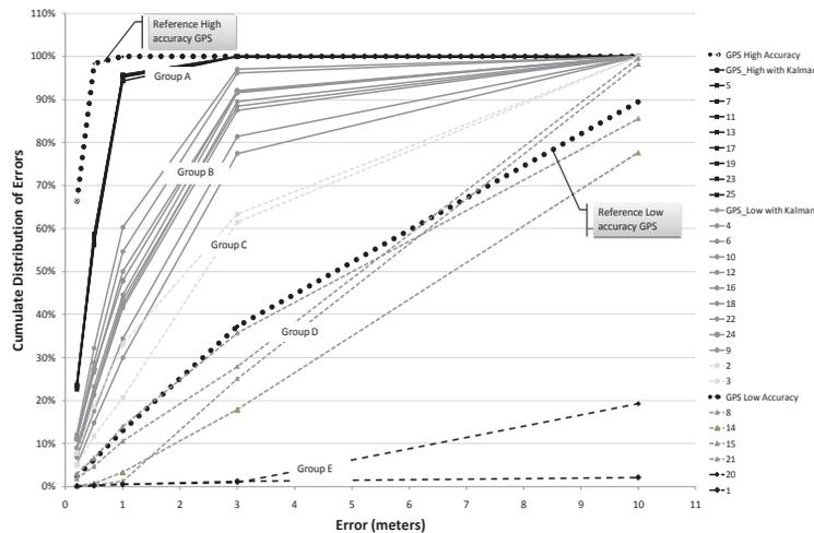
Figure 3 – Error in the positioning of the vehicle
