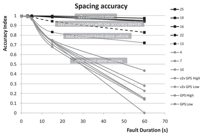
Figure 6 – Accuracy in reproducing spacing in case of both radar and GPS fault
