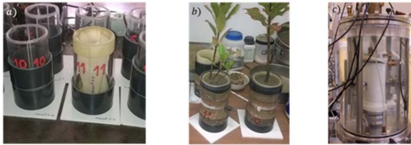
Fig. 2. Pictures of the construction of the moulds (a) and of the preparation of the rooted samples (b), while (c) shows the triaxial cell during the test L1.
