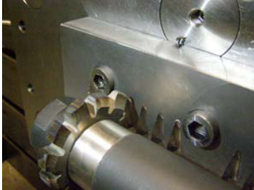
Figure 3: Rack gear cutting with a high speed involute cutter ground to a single tooth.
