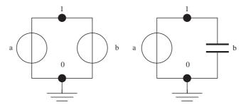
Fig. 2. Left: A loop of voltage sources. Right: A capacitor/voltage source loop.
