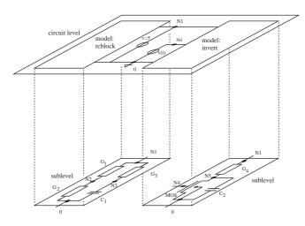
Fig. 3. Example of a parent circuit with two, parallel, sub-circuits.
