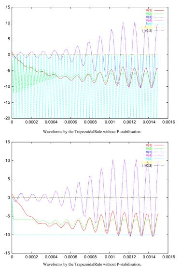
Fig. 4. Waveforms of a circuit with DAE-index 2 obtained by the Trapezoidal Rule without and with **P**-stabilization.
