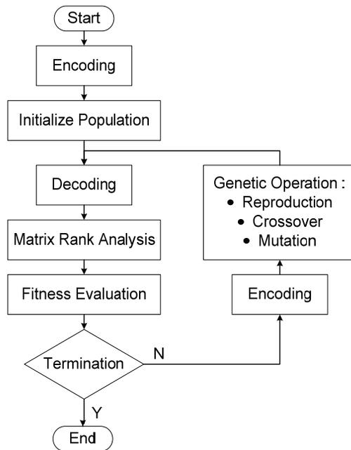
Figure 4: Solution procedure for searching a tensegrity structure algorithm.
