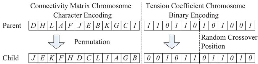
Figure 3: Genetic operation for triplex tensegrity structure example.
