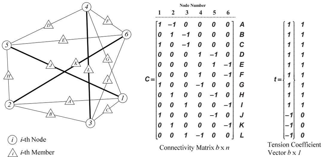
Figure 2: Encoding scheme for triplex tensegrity structure example.
