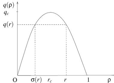
Fig. 2. Fundamental diagram for the flow density.
