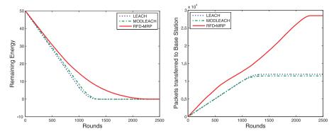
Fig. 3. (a) Remaining energy vs rounds; (b) Number of data packets transferred to base station vs rounds.
