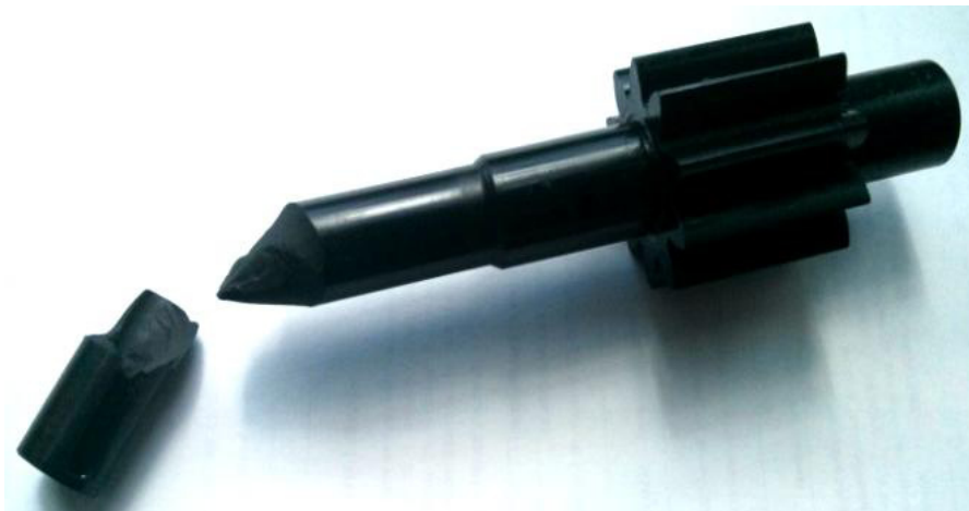
Fig. 3. Breakdown of polymer pinion shaft.
