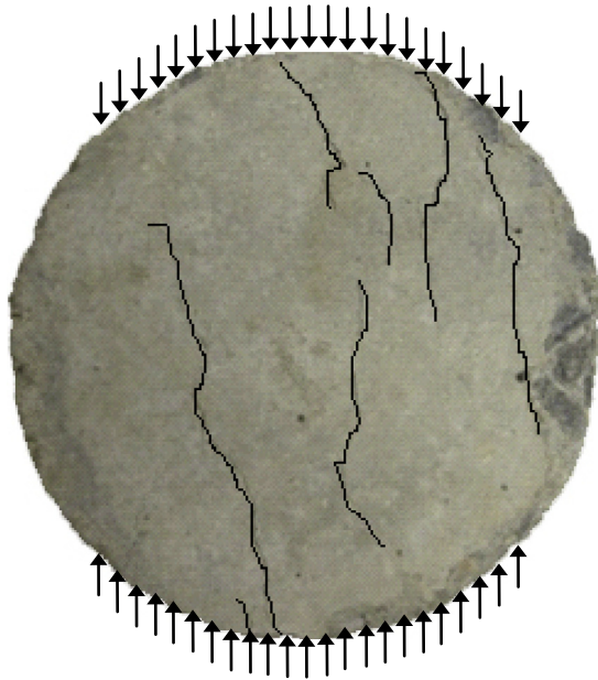
Fig. 3. Typical cracks formed when a core specimen was compressed to failure on its curved surface.
