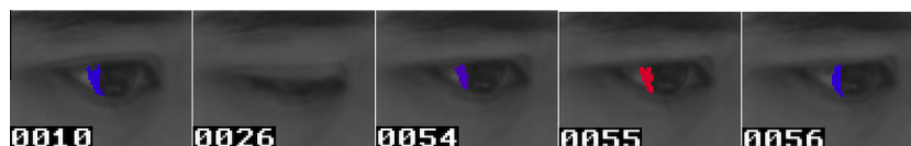
Fig. 5. Video frames corresponding to the data shown in Fig. 6A and B. Frame 10: The eye in a resting phase, as indicated by the cool color. Frame 26: The limbus estimate vanishes during an eye blink. Frames 54–56: The occurrence of OKN, where red indicates a large velocity between frames. A rapid movement to the right occurs over these frames. (For interpretation of the references to color in this figure legend, the reader is referred to the web version of this article.)
